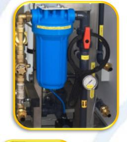
The raw water is microfiltered through a cartridge filter having a 5 micron filtration degree, before moving to the reverse osmosis section in order to protect the osmosis membrane spacers from dirt Downstream of the filter a pressure gauge is mounted that indicates the pressure after the filter, in order to monitor the loss of load on the filter element and its possible degree of dirt.
