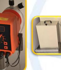
The raw water is automatically drawn from the drinking network by means of the valve and undergoes the constant and proportional addition of a solution of the chemical ANTISCALANT (anti-scaler for membranes) The chemical solution is prepared in the dissolver, and dosed with the dosing
