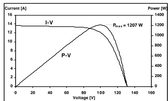
**Fig. 8:** I-V-curves, P-V-curves and MPP power of the array of fig. 7 after cleaning.
