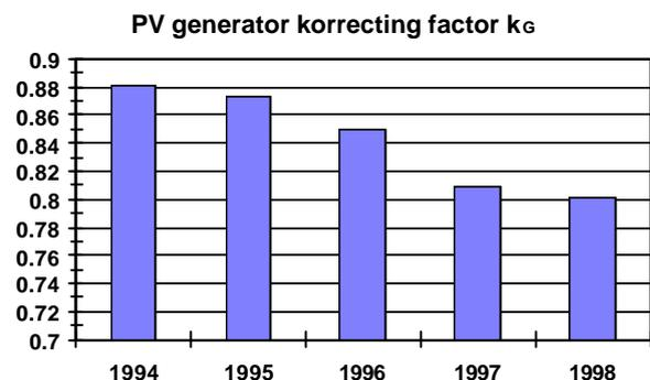
Fig. 9: Generator correction factor  $k_G$  in the 3 summer month in the years 1994 to 1997 and in May 1998.
