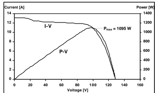
**Fig. 7:** I-V-curves, P-V-curves and MPP power of an uncleaned array (4 parallel strings of 6 modules M55 in series) after 5 years of operation (measured in June 1998).
