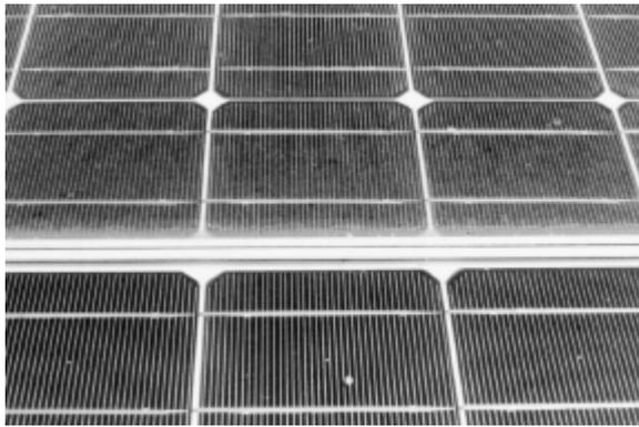
**Fig. 3:** Strip of pollution at lower edge of framed modules M55 (long side mounted in horizontal position, tilt angle 30°) causing partial shading.
