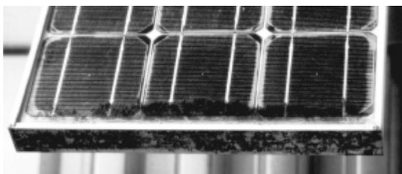
**Fig. 5:** Large strip of pollution at lower edge of framed modules M55 (short side mounted in horizontal position).
