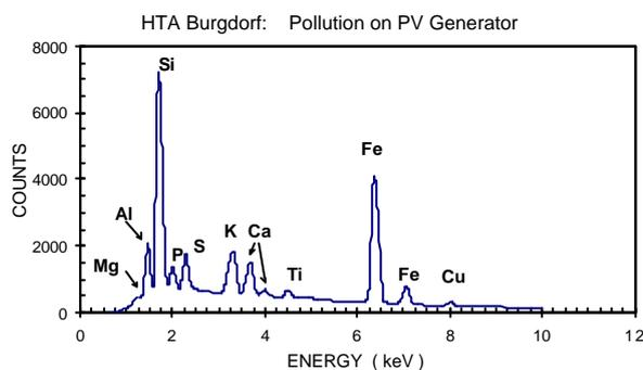
**Fig. 10: Dispersive micro-X-ray analysis of the polluting material showing the most important anorganic components.**
